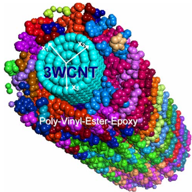
Fig. 1 Atomic structure of a short segment of the 3WCNT + surrounding poly-vinyl-ester-epoxy based effective reinforcement used in the present work
